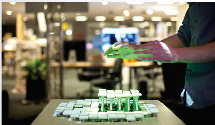
► Recompose: Direct manipulation and gestural interaction with 2.5-D shape display.
