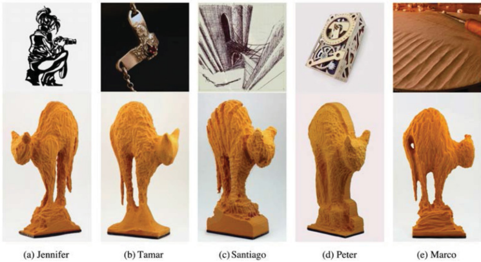
Fig. 13. (a–e) Five cats made by five participants using the FreeD, all using the same CAD model. For each participant, we add an example of prior art.
